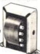
Minimizes line loss and impedance matching problems. Taps at 10, 5, 2.5, 1.25 and 0.62 watts. Accepts 4, 8, 16 ohm speakers. 4 $\frac{1}{2}$ "x5 $\frac{1}{2}$ "x3".
